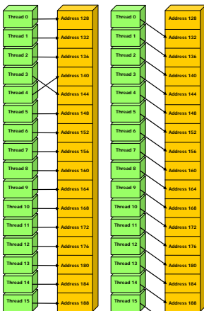
Figure 5-2. Examples of Global Memory Access Patterns That Are Non-Coalesced for Devices of Compute Capability 1.0 or 1.1
