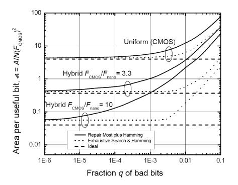
The area per useful bit as a function of single bit yield, for hybrid and purely memories.
